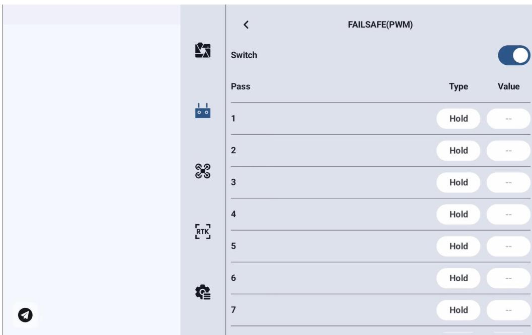
3. The Failsafe Function is disabled by default. The numbers on the left represent the communication channels. When a failsafe output value is not configured, the channel output is displayed as "Hold" by default.
