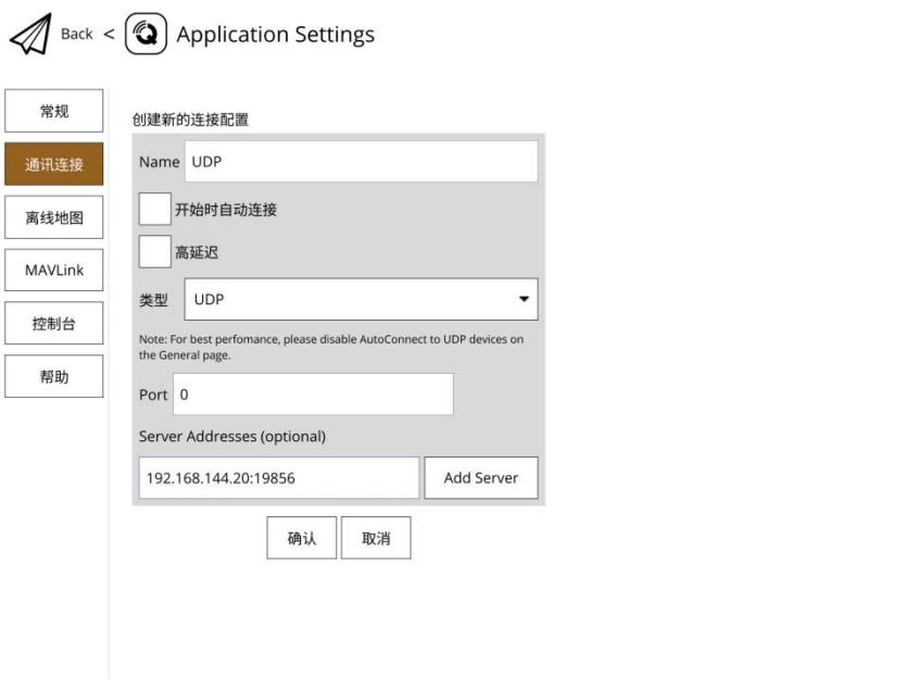
4. Select the configured “UDP” connection and click “Connect”. When the progress bar at the top of the QGC interface starts moving, it indicates that the handheld ground station and the flight controller ground station software are attempting to establish telemetry communication. Once the connection is established, data communication will proceed normally.
